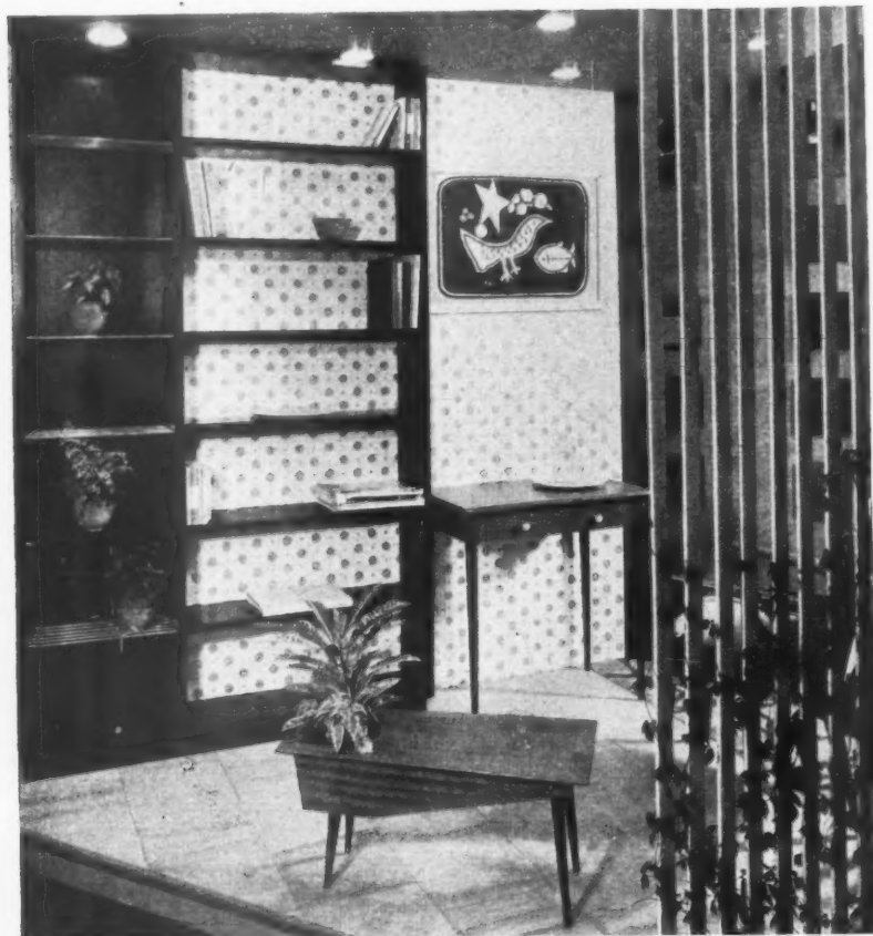
On this stand at the British Plastics Exhibition, Olympia (for the Vere Engineering Co., Ltd.) the designers, Gaby Schreiber and Associates, have made use of the first synthetic timber board to be produced in unlimited lengths and in widths up to 4 ft. This board, shown in use here (veneered) for panelling, floors and furniture, is not yet being manufactured, but is expected to cost about 4d. per sq. ft., at a thickness of \frac{1}{4} in. Above, a living room; below, a ship's cabin.
