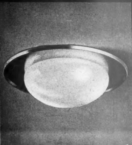
G. 34 CEILING. Backplate. Finishes: Silver anodised aluminium with off-white backplate. Glass: White or ivory flashed opal. Lamps: Up to 2 x 75 watts.
