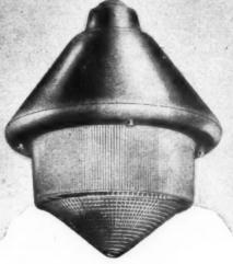
Holophane Enclosed Industrial Units are designed for use where working conditions are such that lighting fittings must be vapour-, dust- and weather-proof while continuing to provide a satisfactory light distribution. The body-casting is constructed of silicon aluminium alloy and the prismatic-diffusing bowl encloses an internal prismatic reflector.
