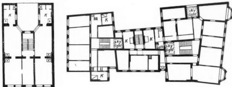
Figs. 1 and 2. Above, left, small flats without corridors at Frankfurt-Oder, about 1895. Above, right, flats with four, five and six rooms. They are built round ventilating shafts with backyards never reached by the sun.
