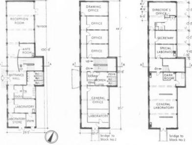
Laboratory block, ground, first and second floors [Scale: 21 = 1' 0"]
