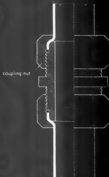
D-D MANIPULATIVE COMPRESSION FITTING: NUT TYPE. (for tubes \frac{1}{4} " to 2" nominal bore)
