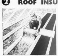
will reduce the loss of heat through a roof-area by at least 70%. This loss, in the average house, is about one-third of all the heat lost in various ways from the structure as a whole.
