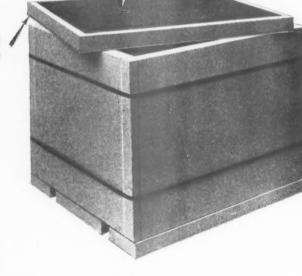
STRAMIT panels for lagging are supplied for large as well as small tanks. When the required sizes cannot be obtained from the standard 4ft. slabs, the required panels are built up at the STRAMIT Works from sections having the meeting edges fitted with "F joints," *i.e.*, tongued and grooved coupling pieces of timber.
