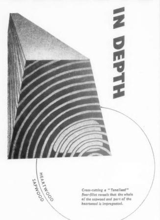
With small sized trees being used more and more to meet the demand for building timber, deep preservation is of vital importance. The sapwood content of timber cut from thinnings is very high and has little resistance to decay. Vacuum/Pressure impregnation plants are sited throughout the country. For details write to:
