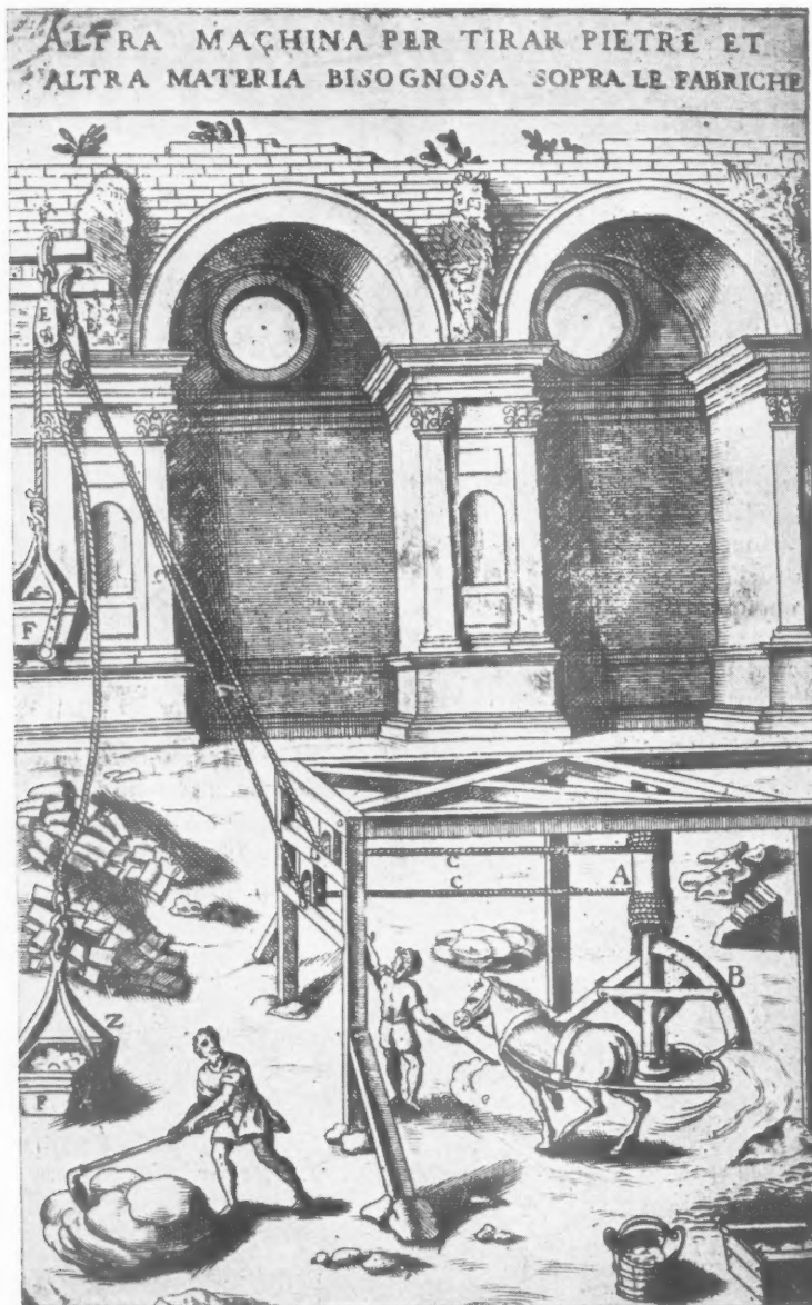
This apparatus is a project for raising stones and other materials for building construction. The prime mover appears to develop one horse power.
