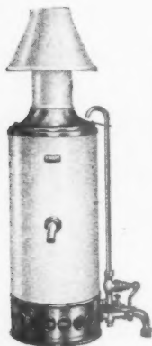
No. 30 Bath Heater. Supplied in a number of finishes with interlocking gas and water cocks or automatic valve. Hot water output 3 gallons per minute raised 40° F. above cold.
