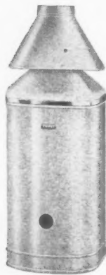
M.210 Multipoint provides an instant and constant hot water supply to Bath, Basin, Sink and other points at a "Turn of the Tap". Hot water output, 3.5 gallons per minute raised 40° F. above cold.
