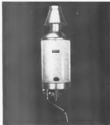
S.140 Bath and Basin Heater. A new design with swivel spout to meet the demand for a low priced bath heater of small dimensions for the modern bathroom. Hot water output, 2.5 gallons per minute raised 40° F. above cold.
