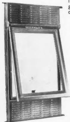
'PERMAVENT' Venti-light Type VAS—all-steel — gauze-backed multi-louvres top and bottom — top-hinged light with locking push-stay—delivered unglazed —permanent ventilation even when closed.
