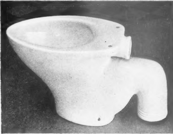
Figure 1. One of the latest developments in lavatory pans (Adamsez), showing, above, a clean-lined and attractive shape (which could be even further improved by corbelling), and left, the rimless bowl. The force of the flush can be adjusted at the inlet, so that the water cleanses the maximum area of the bowl without splashing over the edge. Thus any fouling is immediately detected, instead of forming under the rim, as in normal bowls.
