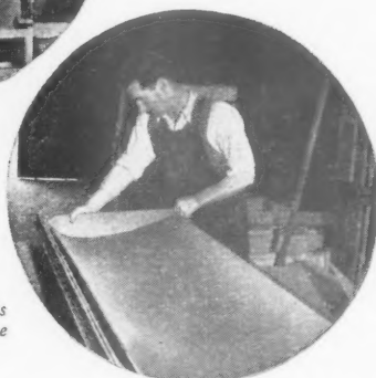
Sundeala boards can be bent to shape
