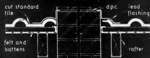
TYPICAL DETAIL AT ABUTMENTS
