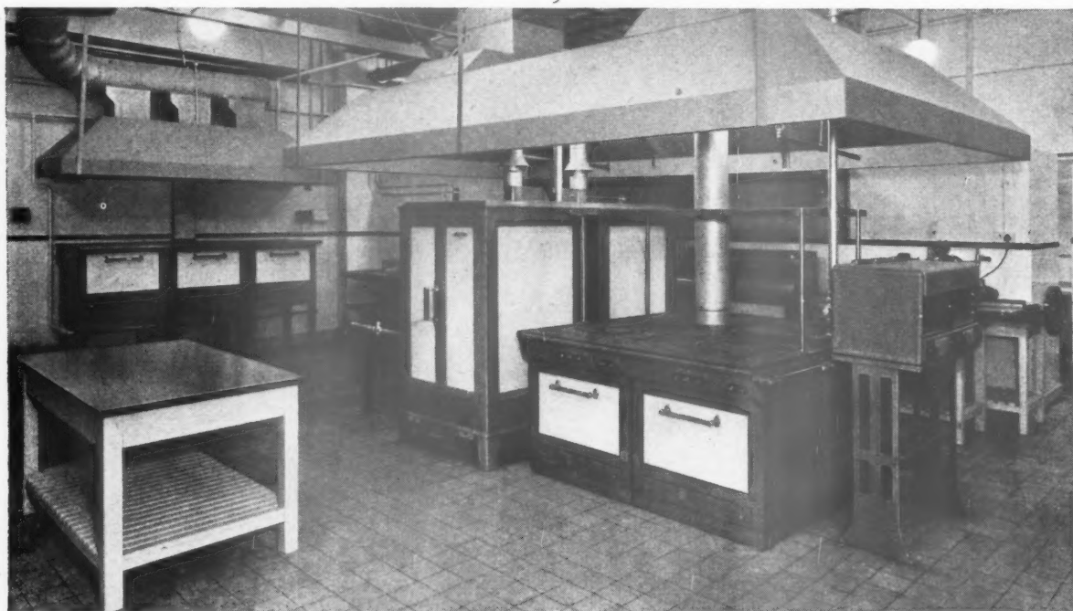
Canteen Kitchen showing 4-oven 701 range, G3 grill on stand, 803 roasting ovens and elevated general-purpose ovens.
