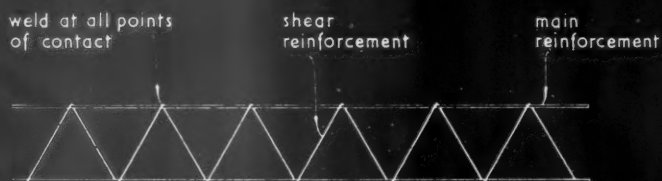
standard unit with nominal shear reinforcement
