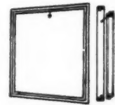
Window inverted for cleaning.
