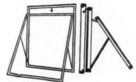
Double glazed window inverted and sashes separated for cleaning. (Outer sash stay hung for wide windows.) Note wide access to the interspace provided by special stays.
