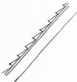
Fig. 8. Tiled pitched roof.—Generally satisfactory. No vapour barrier occurs on the cold side, the joints provide for air and vapour movement and the tiles provide some absorption.
