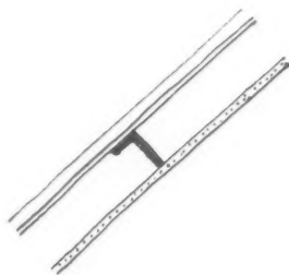
Fig. 15. Sheeted roofs with insulating lining.—A common factory roof: generally satisfactory for normal humidity conditions where no air conditioning and no steam process occurs. It is suitable, for example, for the light engineering type of factory. In higher humidity conditions vapour will penetrate the joints and lining sheeting and often in winter, condense on the underside of the roof covering: it may drip on to the lining and cause trouble. The risk is greater with thin metal roof coverings than with asbestos cement, particularly if with the former the overlaps are sealed and the cavity unventilated.
