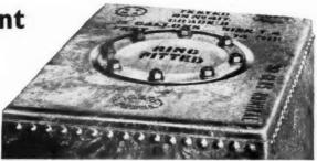
the India Rubber Ring which is supplied with the tank. This ring, together with the grummets fitted under the bolt heads inside the tank, enables a perfect seal to be made in much less time.
