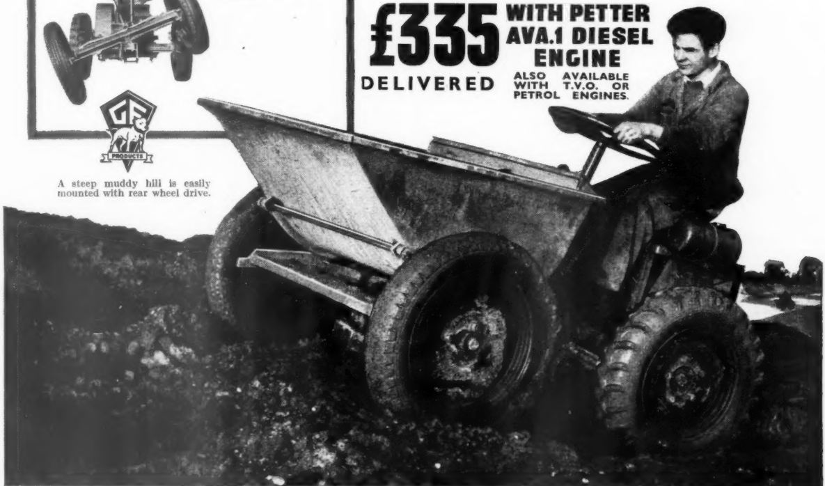
Floating Front Axle. Allowing either front wheel to mount a 16" obstacle.
