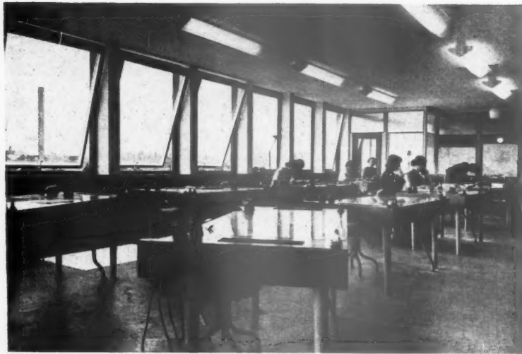
Top and above, two views of the operations room of the Emergency Bed Service for London on the third floor. The floor is covered with cork and the ceiling with acoustic tiles for sound deadening. Left, typical lettable office space below third floor level.
