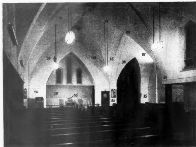
Fig. 8 (top). The interior as it appeared with the original artificial lighting, the figures being "apparent brightnesses." The direct illumination on the vault is too high, with too much light on the left side, giving insufficient modelling. The altar is lost against its dark background.
