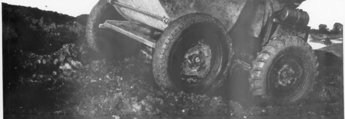
A steep muddy hill is easily mounted with rear wheel drive.
