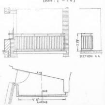
Elevation, plan and section A-A of typical private balcony  $[Scale: \frac{1}{2}" = 1" 0"]$
