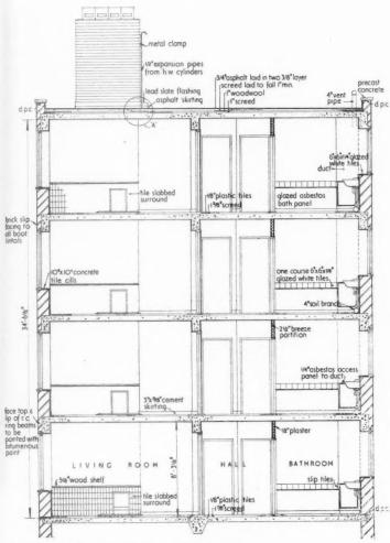
Typical cross section facing south [Scale: 4" = 1'0"]
