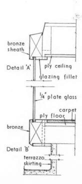
Figs. 6 and 7. Section through fascia and through the window shown in Figs. 4 and 5, (Note: the terrazzo skirting at the foot of the window backs into a 41 in. brick wall not shown in the drawing).
