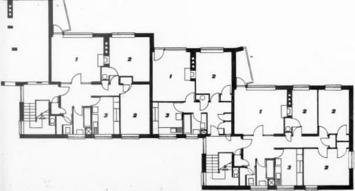
Part third floor plan, showing three types of flat [Scale: 4" = ]1" 0"]
