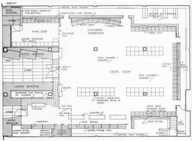
Fig. 1. Layout Plan. Each tinted area represents a separate prefabricated unit.
