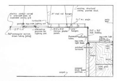
Fig. 13. Section through part of the ceiling and the fitting rooms.
