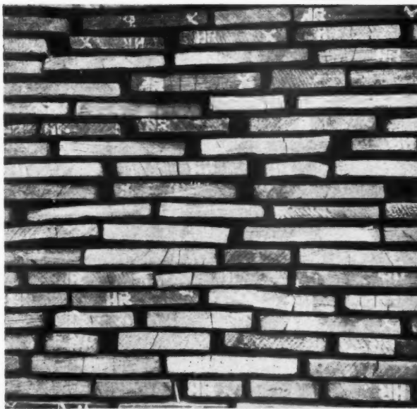
Square edged boards of coigue. The boards are of varying widths, from 4 to 12 inches, but the nominal thickness should be constant. This is an unusually bad parcel of timber, showing shakes, warp, and twist, and emphasizes the importance of careful specification.
