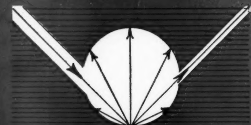
From porcelain or synthetic enamel surfaces: a mixture of diffuse and specular reflection is obtained. See footnote to Table 3.
