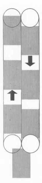
The recent installation illustrated consists of three Paternosters serving seven floors. Each car holds two persons comfortably and is capable of transporting 600 persons per hour in each direction.
