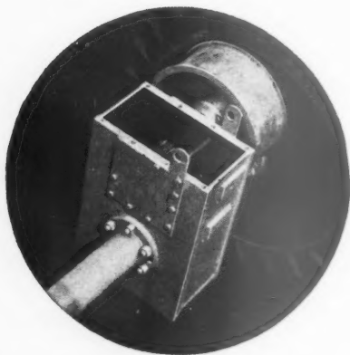
The sturdy Gear Box and Back Axle are specially designed and made by George Fowell for extra heavy duty.
