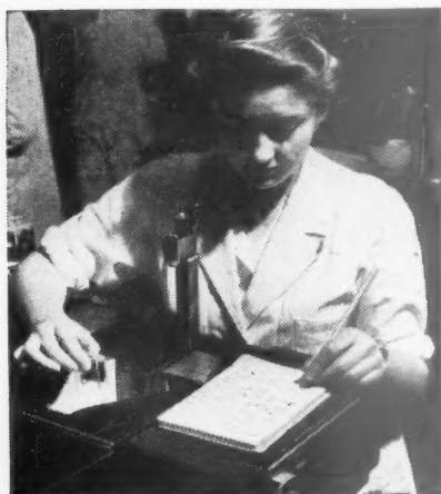
Strength of dye colours being established — by tintometer.
