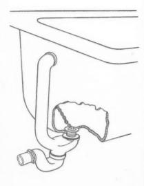
Top, the new Compac bath by Allied Ironfounders; above, sketch showing the combined waste and overflow fitting. Below, a Perkins oil-fired boiler.
