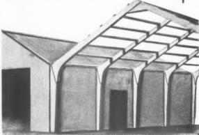
Croft Precast Reinforced Concrete Portal Frames are supplied in standard single or multi spans of 18°0°, 25°0°, 30°0° and 40°0° and if required, with hollow or solid concrete block walls and partitions, "Big Six" asbestos roofing, asbestos gutters and down pipes, steel windows and roof lights to requirements. Particulars and details on request.
