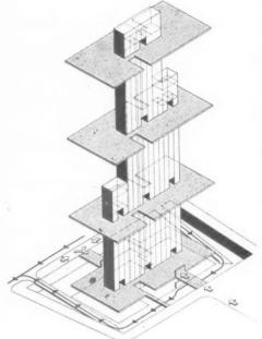
Above, vertical distribution of lift banks. Above left, pedestrian access bridges from street level on the west side. Below, sketch of typical corner treatment on ninth and eighteenth floors, where there is a continuous balcony around the four sides of the block.
