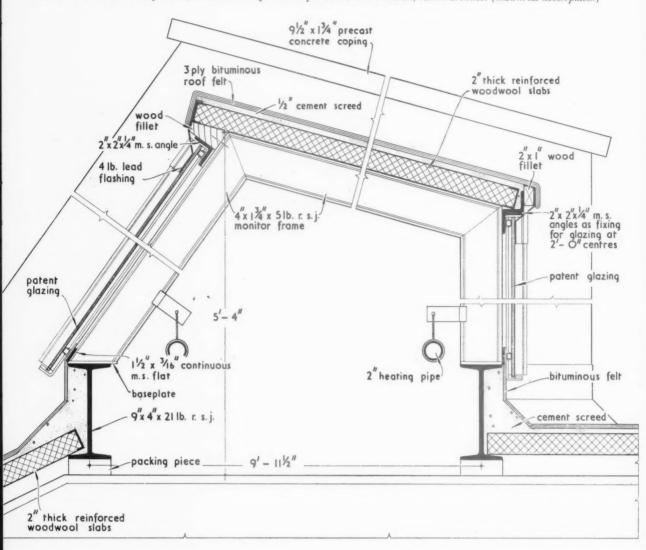
VERTICAL SECTION THRO' MONITOR. scale  $1\frac{12}{2} = 1^{\prime} - 0^{\prime\prime}$
