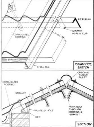
No other building slab possesses ALL these properties As well as being invaluable for reducing heat losses, Stramit confers all the benefits of a low-cost dry construction.  $\bigstar$  It is pre-cut to size to save time on site and to avoid cutting to waste.  $\bigstar$  It has light weight combined with great strength and rigidity.  $\bigstar$  On flat roofs no screeding is required.  $\bigstar$  It has a good fire-resistance classification and a high degree of sound absorption.
