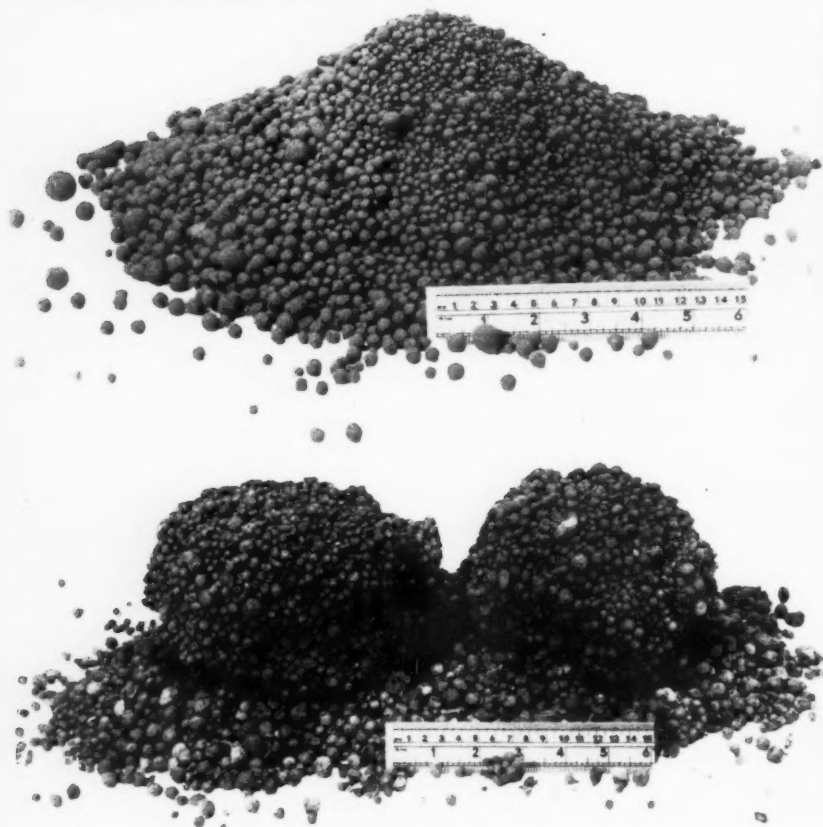
Fig. 1. (top left). Unburnt pellets. Fig. 2. (top right). Pan for pelleting of ash. Fig. 3. (above left). Sintered p. f. pellets. Fig. 4. (above right). Small furnace of refractory concrete. Fig. 5. (right). Large kiln under construction.
