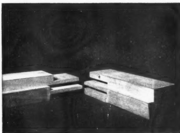
Fig. 16. Above and below. The comb joint as would be used at the corner of a casement window. The slots have been arranged to coincide with the mouldings on the section. The splay to the section in the example below has been made after the joint by the use of a router.
