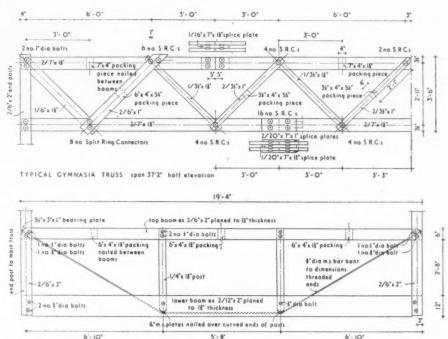
Fig. 13. Details of timber trusses used in gymnasia block.
