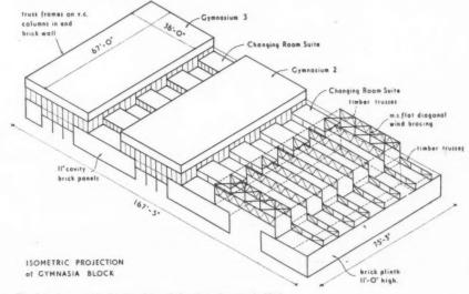
Fig. 14. Axonometric showing the roof planning of gymnasia block.
