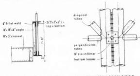
SECTION THROUGH EDGE BEAM PLAN OF BOTTOM BOOM FIXING
