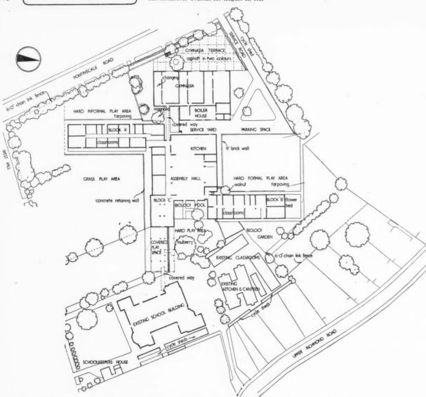
Fig. 1. Layout plan of new buildings showing relationship between Assembly Hall and Gymnasia blocks and the three classroom blocks.
