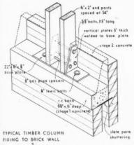
Fig. 12. Axonometric showing the fixing of timber solumns.
