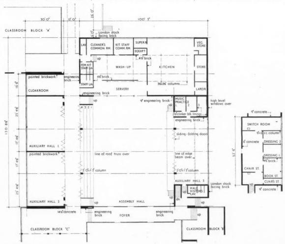
Fig. 2. Plan of the Assembly Hall.
