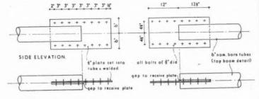
Fig. 7. Space frame jointing details.
