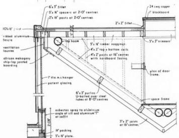
been contrived by roofing consecutive bays from the tops and bottoms of the trusses and fully glazing the change in roof level. The design of the truss has been influenced by the need for daylight and the desire for the minimum of interference from cross bracing.
