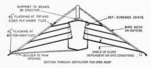
It can be supplied as illustrated for open roofs or with duct and hopper for ceiled roofs. Made in any length in copper, zinc or galvanized steel (painted).
