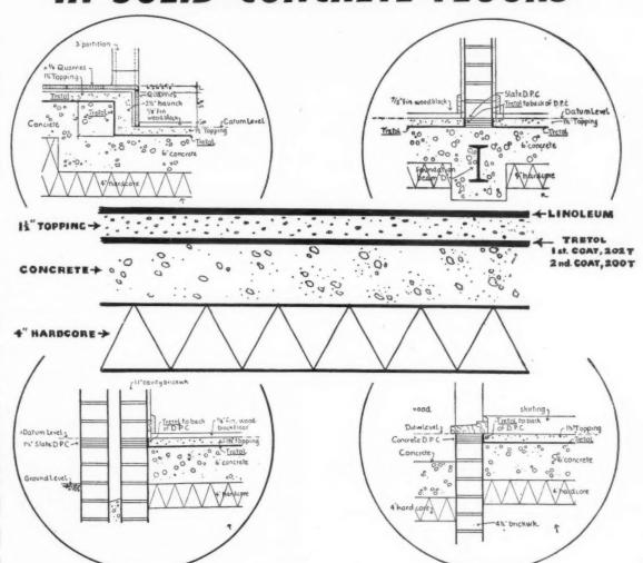
Where ground floors are to receive a floor covering, the use of a continuous Bitumen Membrane is essential. Not only is this necessary to prevent dampness, but also rising moisture vapour, the latter being injurious to most types of floor covering and to health.
