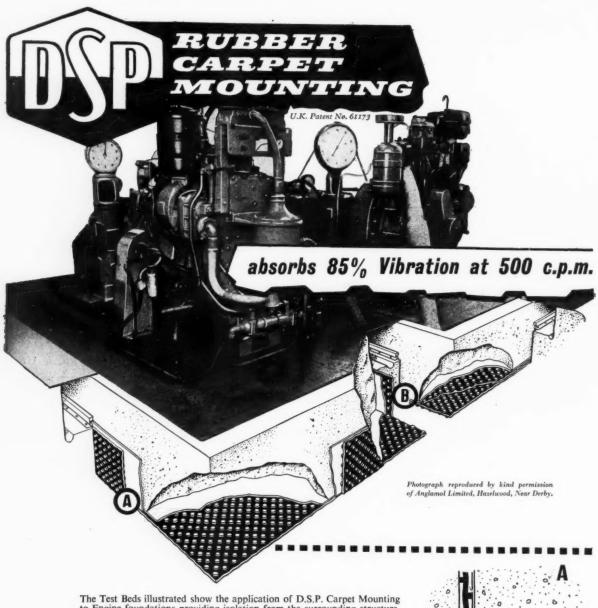
to Engine foundations providing isolation from the surrounding structure. The method of application of the Anti-Vibration carpet is decided by the vibration characteristics of the individual Engines.
