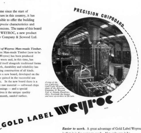
Easier to work. A great advantage of Gold Label Weyroc is that it is far easier to work. Not only can it be speedily and easily cut by means of ordinary hand tools or woodworking machinery, but the tools themselves need sharpening far less often. These tactors simplify production planning and reduce fatigue, accidents and labour costs.
