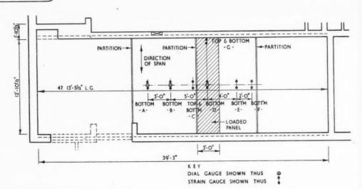
Fig. 1. Plan of the test floor showing position of dial and strain gauges.
