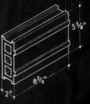
cut on site from stretcher block CUT CLOSERS.
