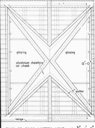
PLAN OF ROOF LANTERN LIGHT. scale 3/" = 1'-0"
