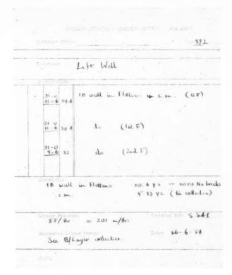
Fig. 1. Typical data sheet taken from a schedule of basic quantities.
