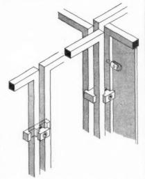
pins which, passing through the two sides of the forked head of the pegs, are punched through the intervening sheet. Finally the frames are held together by a repertoire of chromium plated m.s. clamps, cut from  $\frac{5}{8}$ -in. by  $\frac{5}{16}$ -in. bars which are held in place by socket head screws.
