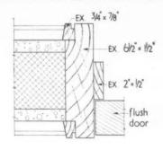
Corner fixing of solid and glazed pre-fab.ic.ited panels
