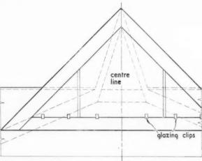
PART ELEVATION OF LANTERN LIGHT. scale  $\frac{3}{6}$  =  $\frac{1}{1}$  – 0
