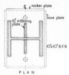
Details of roller bearing to centre stanchions [Scale: I" = I'0"]
