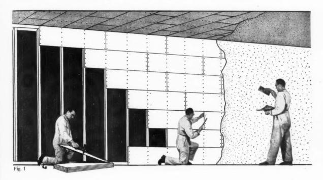
Diagrammatic representation of the correct application of GYPROC Lath
