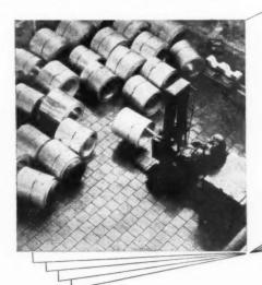
To satisfy the requirements for a non-dusting, level surface, Stelcon Anchor Steel Plates were chosen for the floor of their new Strip Mill by Messrs. Firth Vickers Stainless Steels Ltd., Sheffield.
