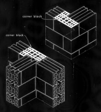
TYPICAL APPLICATIONS OF CORNER BLOCKS. DETAIL OF WINDOW OPENING.
