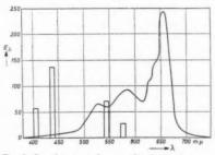
Fig. 2. Complete spectral energy distribution for warm white lamp. Note: the vertical component represents relative energy, the horizontal component shows wavelength.
