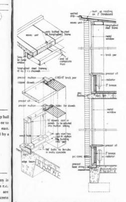
Isometric sketch of p.c.c. facing units to south elevation main classroom block. [Scale: \ \frac{1}{2}" = 1'0"]
