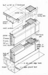
Isometric sketch of p.c.c. facing units to north elevation, main cloakroom block.
