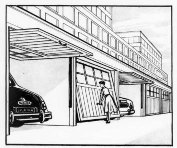
This perfectly counterbalanced overhead gear is designed for those applications where a one-piece door is preferred to the folding or sliding types.
