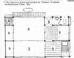
Fig. 3. The plans of two small Japanese houses showing the proportion between fixed walls (heavy lines) and sliding partitions. A Tokonoma is a recess which houses a picture.
