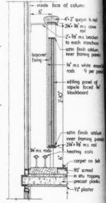
Section through spandrel panel in towe block [Scale: § " = 1' 0']
