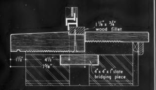
WITH STANDARD METAL WINDOW AND FRAME. (showing Il"cavity wall)
