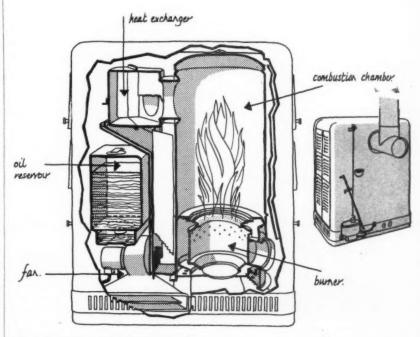
Fig. 4. An American oil burning air heater with fan.
