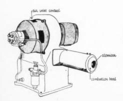
Fig. 1. Left, Doby L4/1 pressure jet burner. Rating 75,000-175,000 B.T.U./hr.
