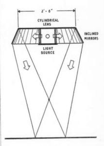
Fig. 2. Diagram showing "scialytique" principle.
