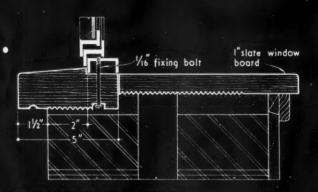
WITH STANDARD METAL WINDOW AND FRAME. (showing II" cavity wall)
