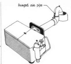
Fig. 3. Nu-way Home Fire vaporising burner. Rating 15,000-65,000 B.T.U./hr.
