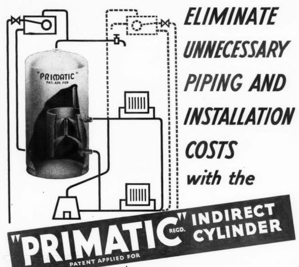
The 'PRIMATIC' copper hot water storage cylinder is fitted in the same way as an ordinary direct cylinder and yet functions as an indirect cylinder. The primary and secondary waters are fed from only ONE cold feed tank, and yet cannot intermix. Radiators can be fitted to the circuit, iron boilers can be used, and the tap water is free from contamination.
