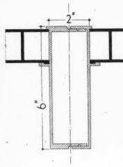
3 ft. 4 in., 4 ft., 6 ft., 6 ft. 8 in., 10 ft., can horizontally, and 9 ft., 10 ft., 11 ft., and 13 ft. from floor to floor. Galvanized straps hold back the frames, slots being provided in both horizontal and vertical planes to are allow fixing tolerances.
