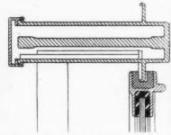
Left, external corner of Quicktho Windowall. Above top: photograph of section of Windowall multion as seen from the outside, but before the aluminium cover strip has been added. Above, section throug Windowall multion showing its division into a central weight-bearing column and two enclosing leaves. Moisture entering the multion will drop down the cavity and pass out at the foot.
