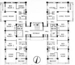
Typical upper floor plan Golden Lane, Finsbury [Scale :  $\frac{1}{24}$ " = 1' 0"]
