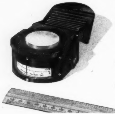
Above: the portable daylight factor meter, designed by the BRS for Evans Electroelenium. Below, one of the range of hand-painted tiles produced by the Queen Elizabeth Training College for the Disabled.
