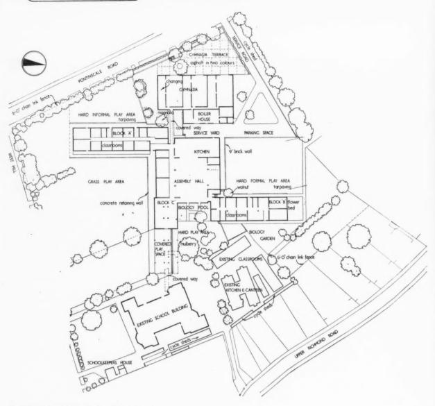
Fig. 1, layout plan of the school and its new extensions. Blocks A, B and C are three-storey blocks and the three gymnasia can be seen at the top of the plan.
