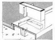
Each mullion spans one floor. The spigot joint leaves the head of the lower mullion free (accommodating thermal movement). The foot of the upper mullion is fixed to a floor slab.
