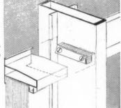
The Wallspan Curtain Wall is completed by windows, fixed glazing and solid infilling panels fixed direct into the grid. It is evident that Wallspan offers remarkable simplicity and speed of construction with a most unusual saving of time and
