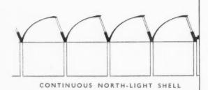
Perfect uniformity of lighting together with the continuity of floor space makes North Light Shell ideally suitable for factory construction.
