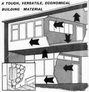
Joining the panels: blocks incorporated in each panel fit exactly. No glueing or nailing.
