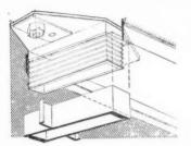
The head of the topmost mullion rides on a spigot bolted to the structural frame. The grid top is completed by head members fixed between the mullions.
