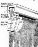
HARDWEARING NYLON gliders slide noiselessly in silicone-treated aluminium rails which can be countersunk or screw-fixed. Twenty different types of rail are available to meet every structural requirement.
