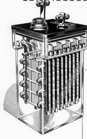
The P.& G. Closed Top Cell has a lid of moulded Dagenite composition with a rubber joint ring, and rubber gaskets between the terminal pillars and lid, to render the lid acid-tight
