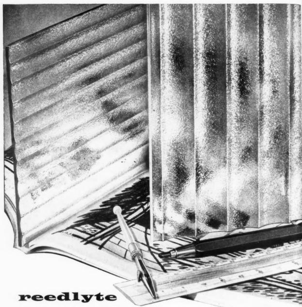
Reedlyte has the simplicity of Reeded glass but, one surface being stippled, a high degree of obscuration is imparted. Reedlyte is used for windows, partitions, and for borrowed lights where considerable, but not complete, obscuration is required and where ease in cleaning is an important factor.
