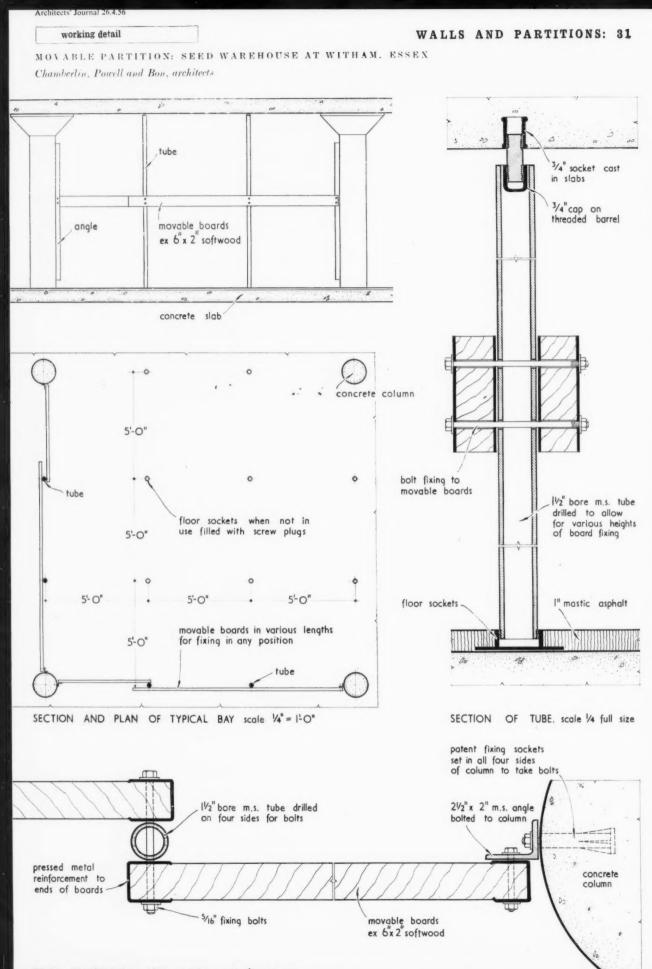
PLAN AT COLUMN AND TUBE. scale 1/4 full size
