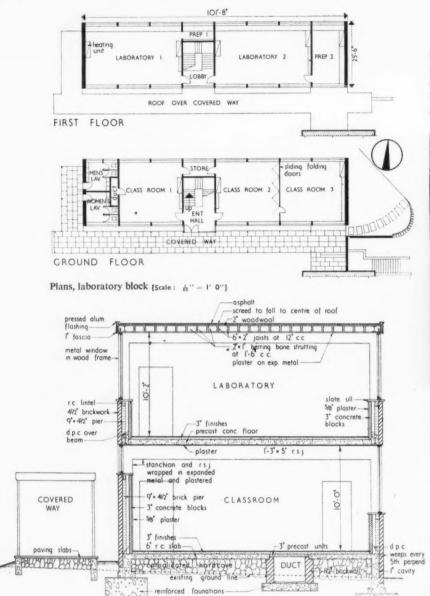
Typical cross section [Scale : #" = 1' 0"]
