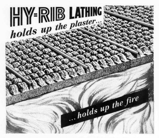
The plaster of a suspended ceiling is a remarkably effective fire baffle while it remains anchored to metal lathing. The three-dimensional mesh of Hy-Rib Lathing is designed to hold the pricking-up coat of plaster in position during the most severe fire.
