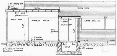
Section I-I through link block [scale : , " = 1' 0"]
