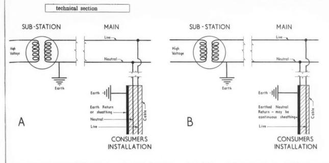
Diagrams showing the connection between consumer's installation and sub-station A (on the left) according to present practice and B (on the right) when "multiple earthing" is used. In B the consumer earths his neutral line, using the cable sheathing for this purpose, thus saving on wiring. For simplicity's sake single wires have been shown on the diagrams but the majority of installations in this country are three-phase, requiring three live wires.
