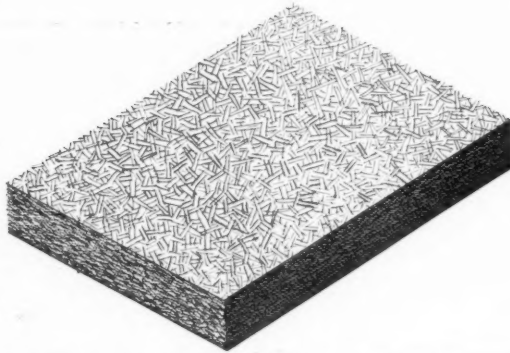
Chipboard: consisting of wood chips bonded under pressure with resin glues.
