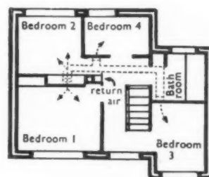
Fig. 5. Warm-air heating system for LCC house.
