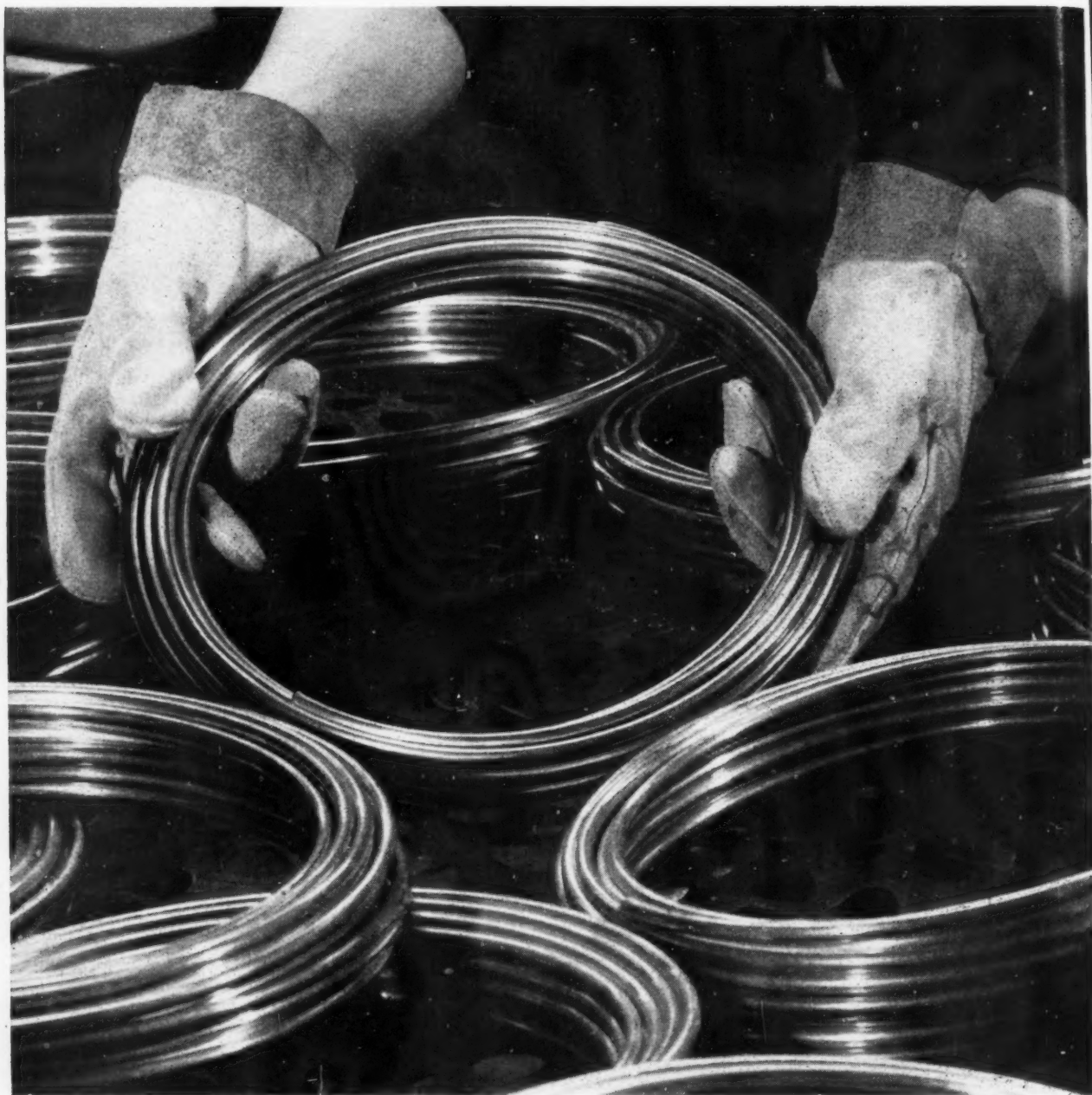
Part of specialised production of coils for refrigerators.
