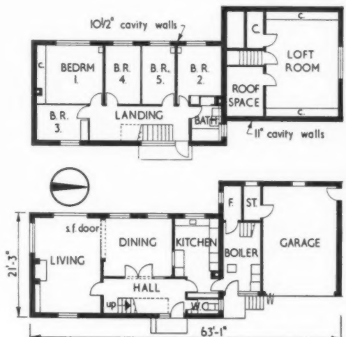
Above: the house at Rickmansworth. Below: ground and first floor plans [Scale: \frac{3}{4} " = 1' 0"]
