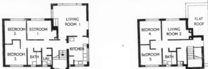
Above left: the house at Reigate. Left: ground and first floor plans. [Scale: \frac{3}{8}" = 1' 0" ]
