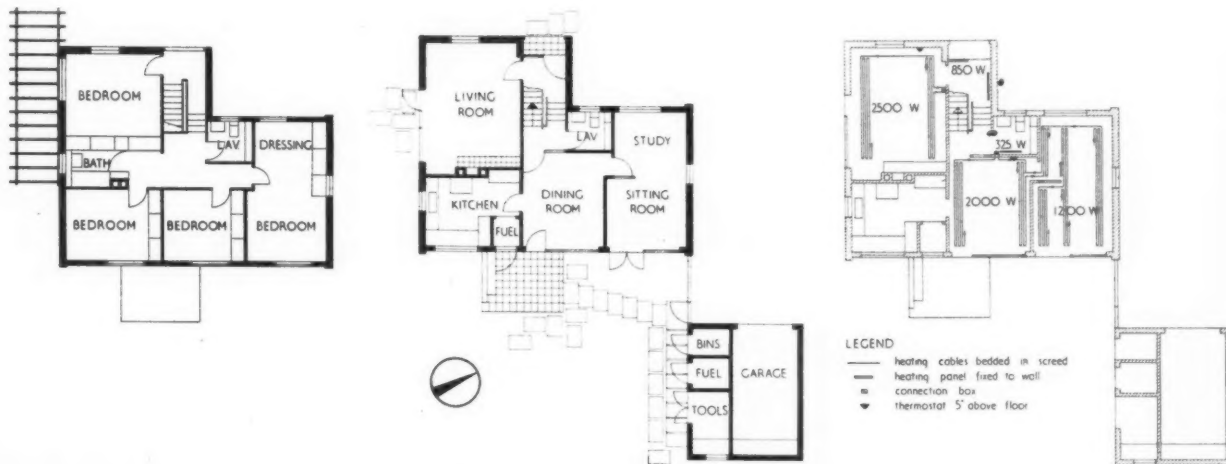
Above: the house at Whiteleaf. Below: ground and first floor plans and, below right, layout of the heating installation. [Scale: \frac{1}{2} " = 1' 0"]
