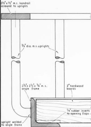
DETAIL OF HANDRAIL. scale 1/2 full size
