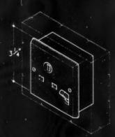
flush switch socket outlet no. 4527
