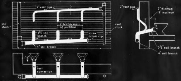
RANGE OF W.C'S ALONG EXTERNAL WALL-EXTERNAL PIPEWORK.
