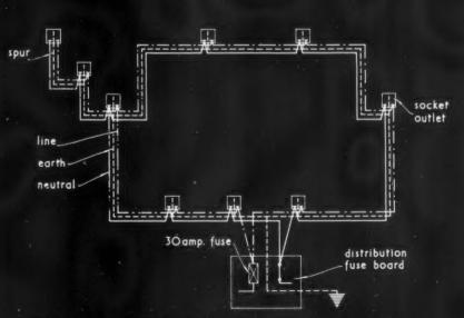
DIAGRAM OF TYPICAL RING MAIN CIRCUIT.
