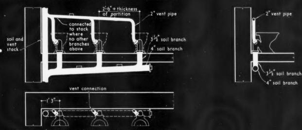
RANGE OF W.C'S ALONG EXTERNAL WALL-INTERNAL PIPEWORK.
