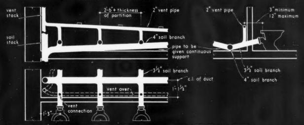
RANGE OF W.C'S AT RIGHT ANGLES TO EXTERNAL WALL- INTERNAL PIPEWORK IN DUCT.
