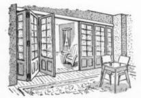
**CENTRE HUNG VEE GEAR** is very suitable for interior use in private residences and public rooms. On the No. 600 VEE gear shown the fittings are not visible on either face of the leaves.
