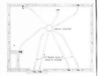
Plan of heating ducts
