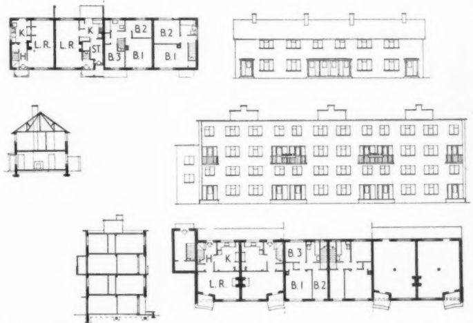
LAYOUT B, MIDDLE. Density: 99 persons to the acre, net. A little to the north-east of layout A, this area, now nearly complete, represents a more urban design-approach. For the purposes of the density calculation, the housing within the broken line was excluded. Below, plan, section and elevation of a typical house and maisonette block. The siting of the semi-detached houses, bottom, makes good use of the land (see layout plan above) and creates a foil to a long maisonette block opposite.
