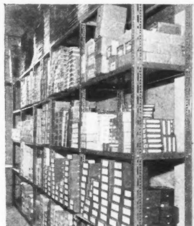
Complete reorganization of busy wholesale department at H. J. Ryman Ltd., Stationers and Printers. Dexion 225 slotted angle and new shelves make the most of cubic space and facilitate handling of materials. Installation designed and erected by Dexion Ltd.
